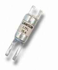
Lawson type "LTFL" are used with current transformer trip release coils on circuit breakers. They are covered by Technical Specification 12-6 published by the Energy Networks Association. They are intended to protect distribution transformers with rated powers from 200kVA to 1,500 kVA.
